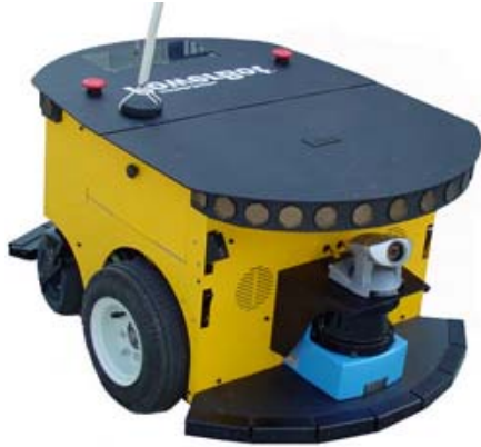
Figure 7. PowerBot carries over 100 ka of payload.
